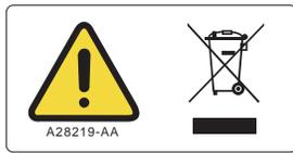
This symbol is required in accordance with the Waste Electrical and Electronic Equipment (WEEE) Directive of the European Union. The presence of this marking on the product indicates:
