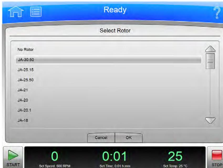
To select a type of rotor for a run program, select the **Rotor** button on the [New Program Page](#) or the [Edit Program Page](#) to display the **Select Rotor** page (Catalog). This page displays the complete list of rotors that can be used with the Avanti JXN series.
