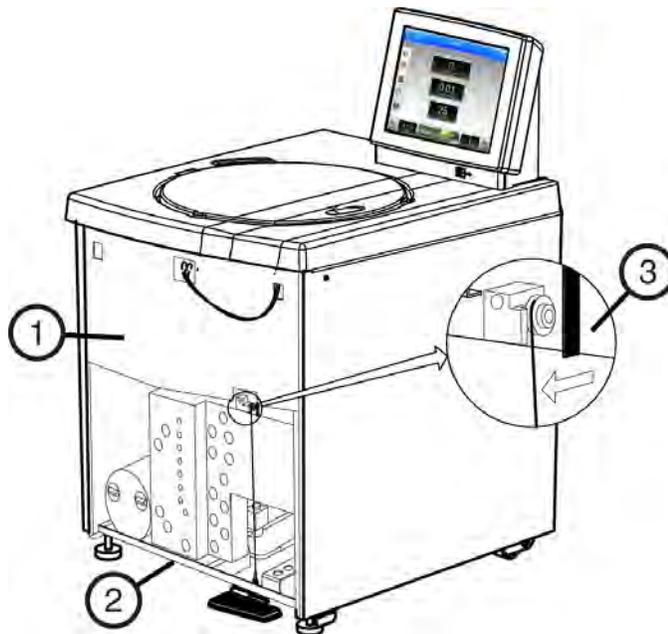
1. Inner Front Panel      3. Manual Door Release Interlock Lever
