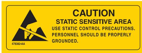
Indicates an area of the instrument which is sensitive to static electrostatic discharge (ESD). To prevent damage due to electrostatic discharge, always wear a properly earth-grounded wrist strap while operating this instrument. For details on proper grounding, see IEEE standard P1100.
