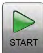
The **Start** Button begins a run with the current settings. Use it only after you have set the parameters for the run.
