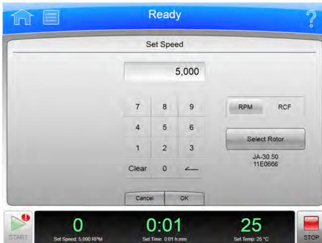
To set the speed for the next run or change the speed of the run in progress, select the **Set Speed** Display/Button on the [Home Page](#) or the Footer Bar to display the **Set Speed** page. You can select the **RPM RCF** button to set the value in RCF (Relative Centrifugal Field) instead of RPM.
