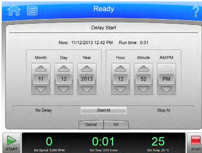
To set a future start or end time for the next run, select the **Delay Start** button on the [Set Time Page](#) or the [Set Speed  \$\omega\$ t Time Page](#) to display the **Delay Start** page.
