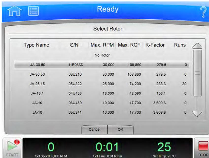
To select a rotor for the next run, select the **Rotor** Display/Button on the Home Page or the **Select Rotor** button on either the [Set Speed Page](#) or the [Set Speed  \$\omega\$ t Time Page](#) to display the **Select Rotor** page. This page displays the library of rotors that have been entered for your instrument.
