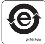
This label indicates that the electronic information product does not contain any toxic or hazardous substances. The center “e” indicates the product is environmentally safe and does not have an Environmentally Friendly Use Period (EFUP) date. Therefore, it can safely be used indefinitely. The circling arrows indicate the product is recyclable. The date code on the label or product indicates the date of manufacture.
