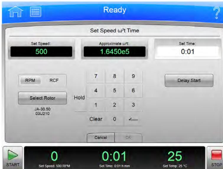
When the  $\omega^2t$  mode is active and you select either the **Set Speed** button or the **Set Time** button on the [Home Page](#) or the Footer Bar, the system displays the **Set Speed  $\omega^2t$  Time** page. The  $\omega^2t$  value is computed from the time and RPM (or RCF) values you enter. Use this page to set the values for the next run that produce the desired  $\omega^2t$  value.
